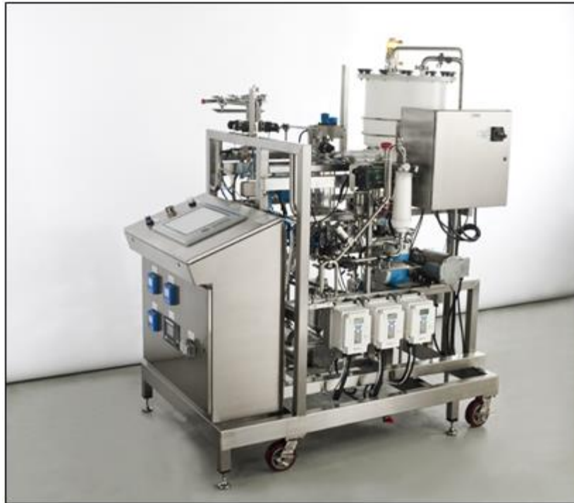
Figure 11-9. Example #1 of modern automated chromatography system (courtesy Pall Life Sciences)
