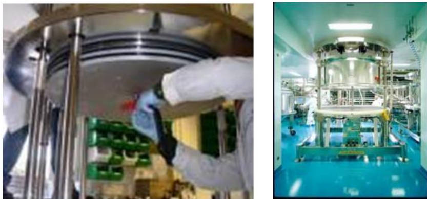
Figure 11-16. Performing column preventive maintenance (without overhead hoist/crane) enabled by the column's integrated hydraulics (courtesy Pall Life Sciences)
