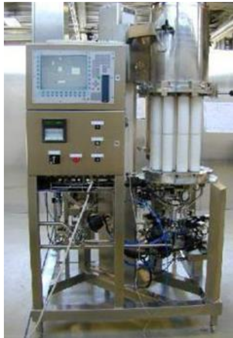
Figure 11-2. Pall Life Sciences Ultipor ® Direct Flow Filtration (DFF) cartridges of various scales (top) and typical automated process DFF system fitted with a multi-round assembly of cartridges in a single housing—partially lifted from its base to expose the cartridges (bottom)—courtesy Pall Life Sciences
